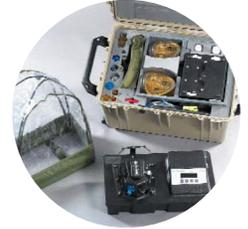
A leakage isolation test allows the operator to isolate the location of a leak and possibly remedy the situation; thereby permitting the continued fielding of the mask. Mask components that are prone to leaks include: voicemitters, exhalation ports and disks, inlet port seals, and drink hoses and couplings.
