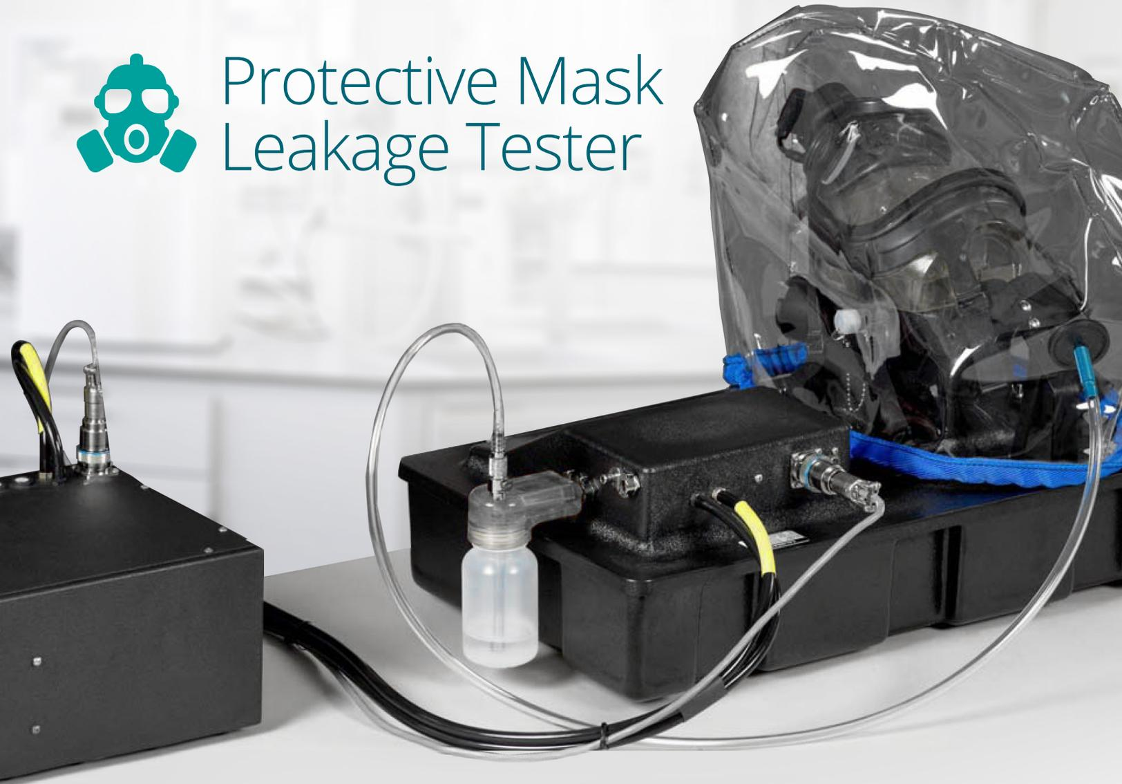
**When donning a protective mask, you deserve the utmost confidence in your gear.** Air Techniques International's Protective Mask Leakage Tester (PMLT) is an aerosol & photometry-based instrument designed to confirm mask seal and integrity as well as individual fit. The PMLT is portable, easy to use, sets up in minutes and provides a variety of mask testing options.
