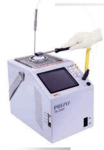
A specific insert, with a reference sensor allowing the temperature control and measure just below the surface, has been developped to calibrate your surface sensors.
