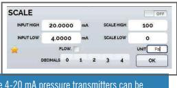
The 4-20 mA pressure transmitters can be calibrated showing directly the scaled pressure that will be displayed jointly with the measured current value.
